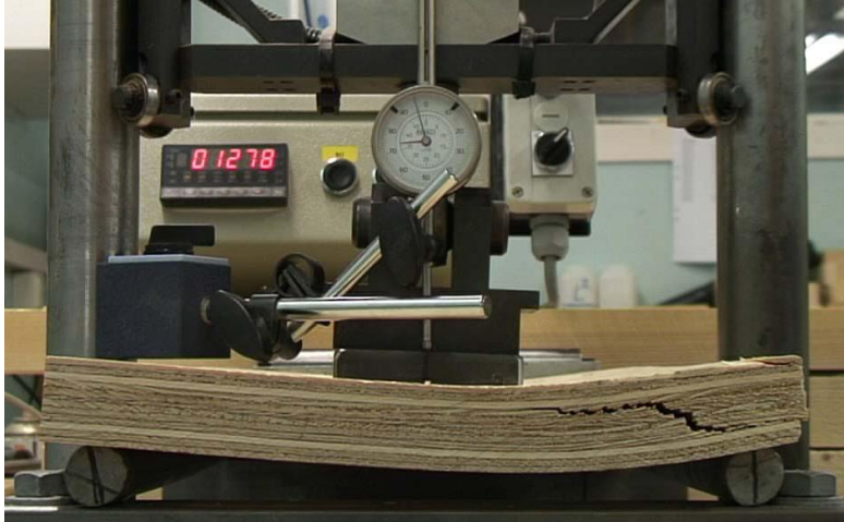
Figure 9: typical failure due to "rolling shear" in a cross laminated veneer lumber plate.
